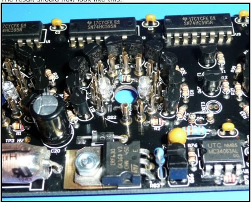
Now put the spacers for the glow lamps over the glow lamp leads and solder them to the PCB. The 2
