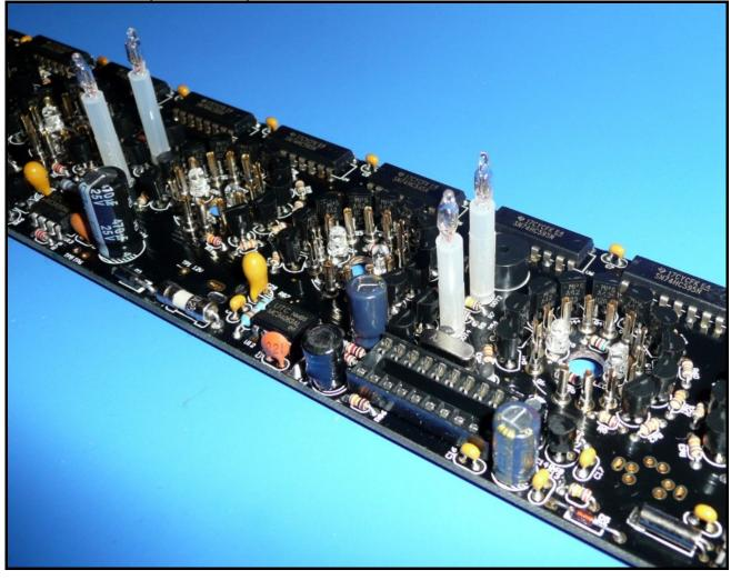
Now solder the 3 switches, the power connector and the PS/2 connector at the other side of the PCB. The result should now look like this:
