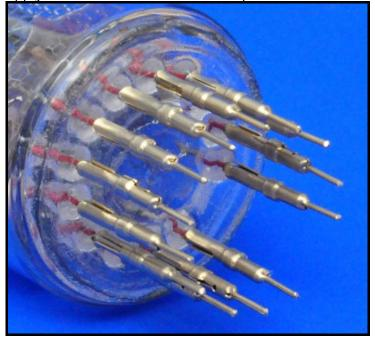
Insert the tubes one after another with the contacts into the drills of the board and align the tubes right-angled to the board surface. Solder the contacts carefully **from the bottom side**. Don't use too much solder, otherwise the solder may flow into the inner side of the contacts. Cut ONLY the thin part of the contacts. Then pull the tubes out of the sockets again.
