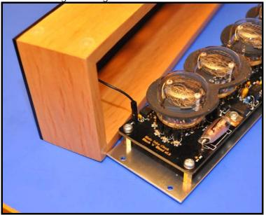
Mount the PCB assembly with the 4 self tapping pan head screw, 2.9×9.5 mm on the wooden frame:
