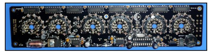
Solder the LEDs to the board. The polarity of the LEDs must be observed! (anode and cathode). The long lead is the anode; the short lead is the cathode. The polarity of the LEDs must match the print on the board!
