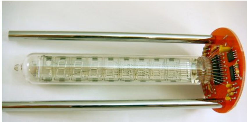
Tube aligned and soldered to the tube pcb.
